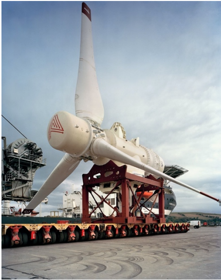
© Luca Sage/FotoDocument The Atlantis AR1500 tidal turbine ready for load-out onto the installation vessel. Nigg, Scotland, October 2017.
